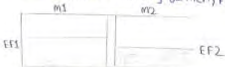
Fig: 11.2: two metal junctions, separated by a thin insulating barrier.
